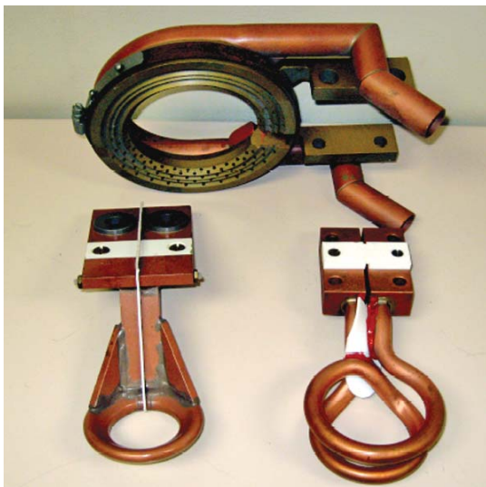
Fig. 1. Typical induction-scan hardening inductors and quench ring
