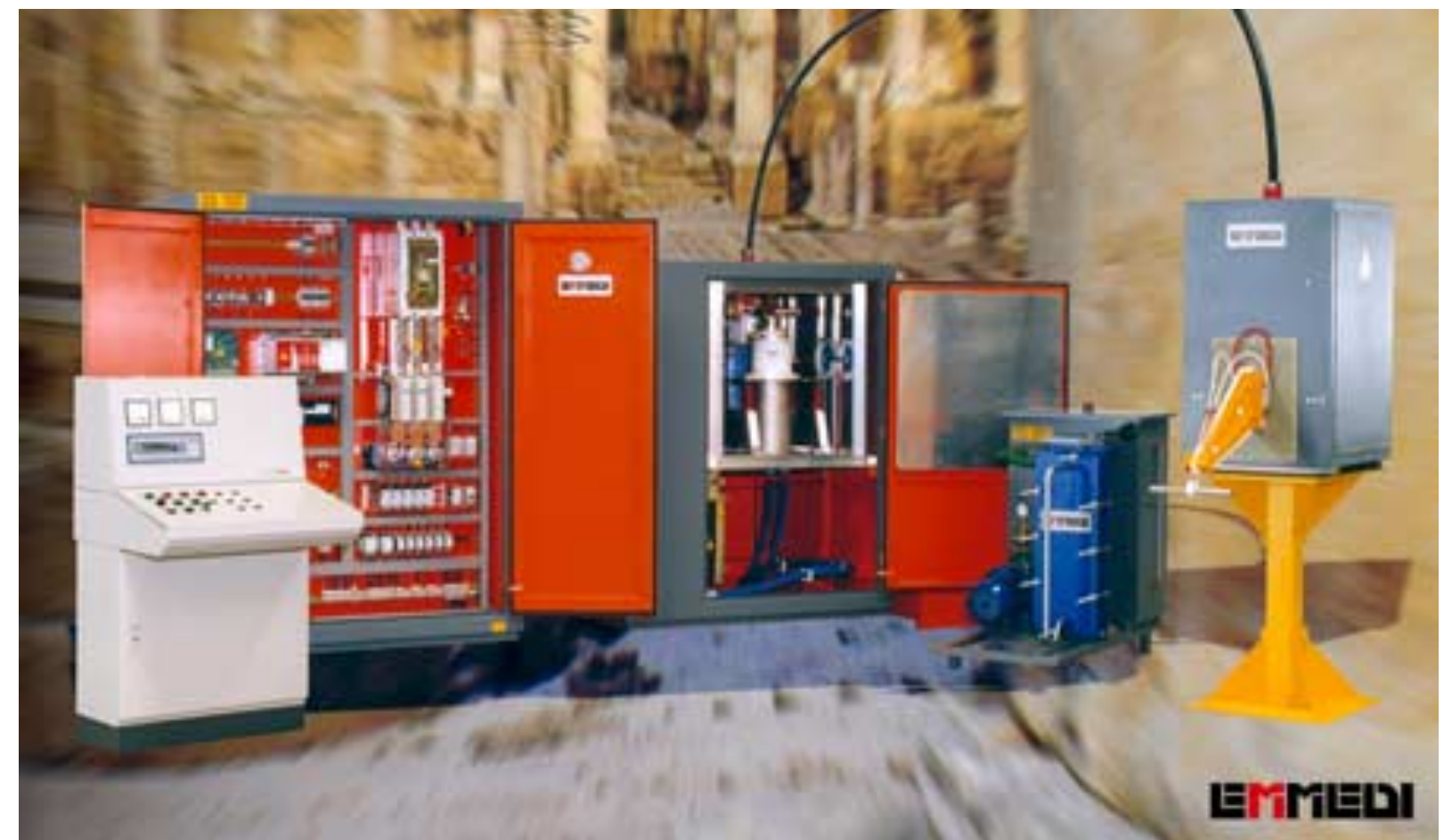
Welder with vacuum tube oscillator, EMMEDI company
